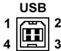
Figure 3-6: USB Connector pin orientation.
