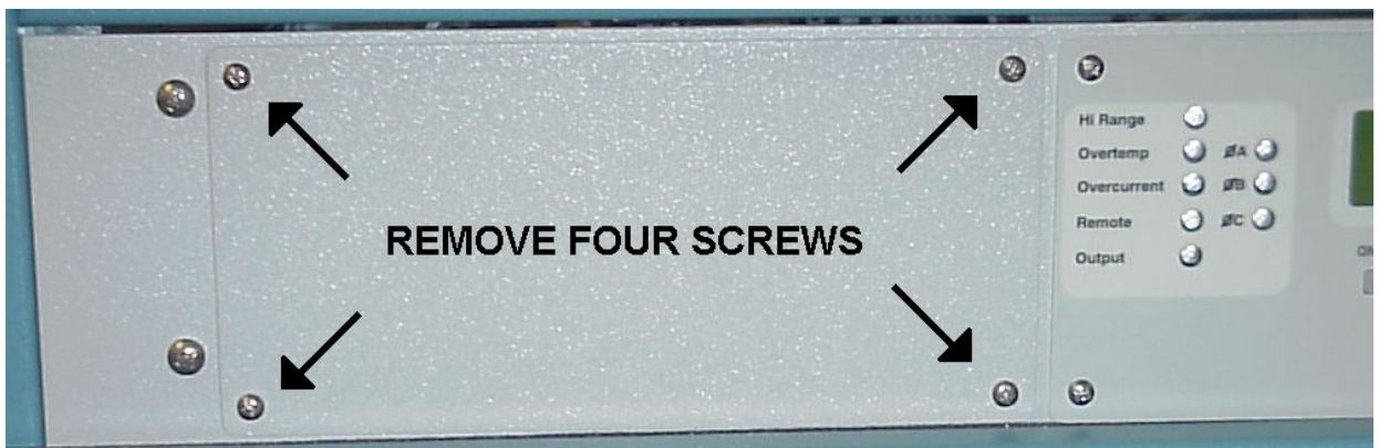
Figure 6-2: Current Limit board access panel
